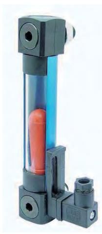
**LV**@ight level gauges allow the sight reading of the fluid level through a transparent tube connected to the tank. O-Ring are located in all joining points to allow a perfect sealing even when the unit is mounted on a non perfectly flat surface.
